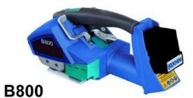
BATTERY POWERED PLASTIC STRAPPING TOOL ADJUSTABLE TENSION UP TO 800 POUNDS 5/8-3/4 INCH WIDTH STRAPPING 16 V 5 AMP BATTERIES
